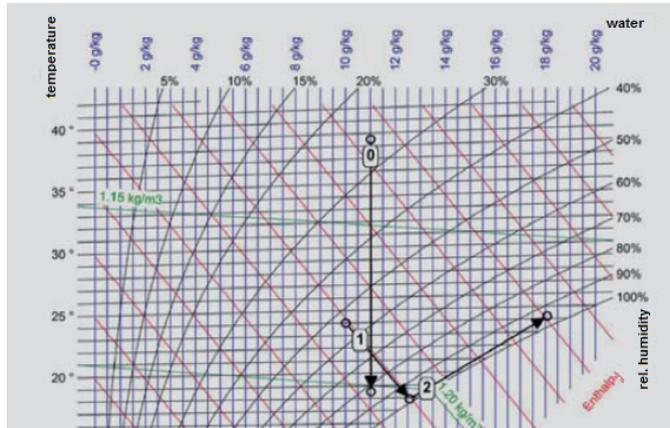
The curves shown in the h,x-diagramme comply to the following measured values:
